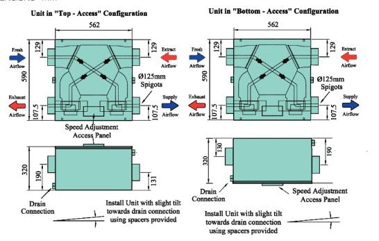
N.B a clearance of at least 200 mm should be allowed on each side of the cabinet for access to the interior
